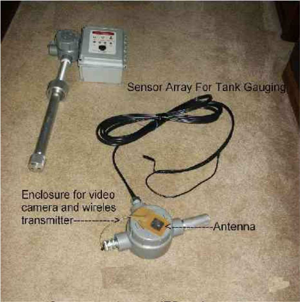
Figure 16- A test unit for wireless communication
